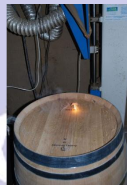
The barrels are marked using a laser gun.
