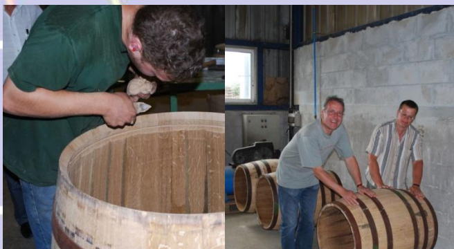
The base of the barrel is fixed in place using a glue made of water and wheat flour.
