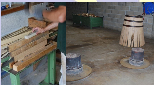
Making the lids and bases – watertightness is ensured by the use of reeds inserted between the staves.
